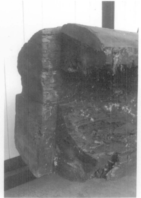
Figure 5. Deterioration occurred between the support post and the hollowed back of the totem. Coal tar had been applied in the past to the hollowed back of this totem to deter fungal decay.
